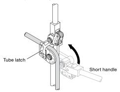
3. Pull the **tube latch** off the tube and remove the tube from the bender groove.
