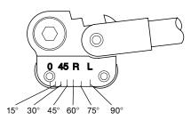
Note: View the marks on the hand tube bender as a 0 to 90° scale when bending other angles.
