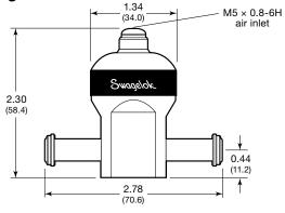
Four mounting holes, M5  $\times$  0.8-6H thread, 0.25 in. (6.4 mm) deep, located 45° from center line, on a 1.00 in. (25.4 mm) bolt circle. M5  $\times$  0.8-6H holes are compatible with 10-32 mounting screws.
