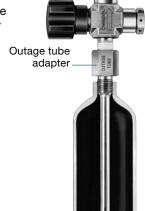
Outage tubes can also be welded directly to the male inlet of a Swagelok nonrotating stem needle valve. The valve is then threaded into the female port of a sample cylinder.
