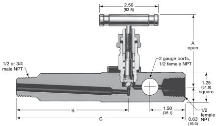
**Ball-Tip Design Valve with Lagging Extension Body**
