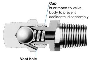
Vent hole bleeds excess liquid or gas from system lines
