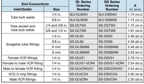
Dimensions shown with Swagelok tube fitting nuts finger-tight.
