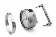
Stainless steel panel-mount clamps are available for flush mounting Swagelok industrial gauges. The panel-mount clamp is easily installed on the gauge. This option is not available on lower mount or S model gauges. Panel-mount clamps on M model gauges must be factory installed and are available as accessories for field installation on B, C, L, and P model gauges.
