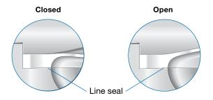
Line seal maintained during cycling of valve. No entrapment areas created.
