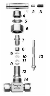
▲ To increase service life, ensure proper valve performance, and prevent leakage, apply only as much torque as is required to achieve positive shutoff.
