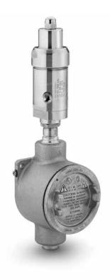
The KEV series is an electrically heated vaporizing regulator with a low internal volume. It can be used to vaporize liquid samples or to preheat gas samples to prevent them from condensing. It features a heating element that is in direct contact with the process fluid for maximum thermal efficiency and is removable for easy cleaning. The KEV regulator has an integral temperature controller and is rated for use in hazardous areas, as identified below.
