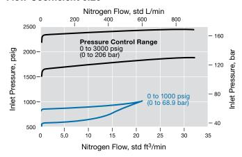
The graphs illustrate the change in inlet pressure as the flow rate increases.
