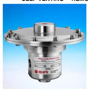
A ratio regulator is a dome loaded pressure regulator. The pilot pressure is usually a 0 - 6 bar signal. Whereas in a true dome loaded regulator the ratio between pilot (=dome) pressure and outlet pressure is 1:1, the ratio in this regulator can be almost anything.
