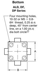
② Bodies with N flow path designator have no mounting holes.
