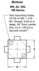
① Bodies with L or R flow path designators have mounting holes reversed from the pattern shown. Bodies with N flow path designator have no mounting holes.
