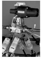
Pneumatically actuated fire series ball valve set up for burn.
