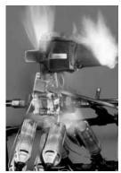
Actuator lubricants begin to burn off, and actuator begins to melt.
