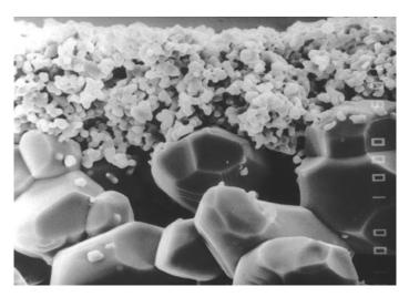
A scanning electron microscope image shows the two membrane layers of the filter: ultrafine and fine (as shown from top to bottom).
